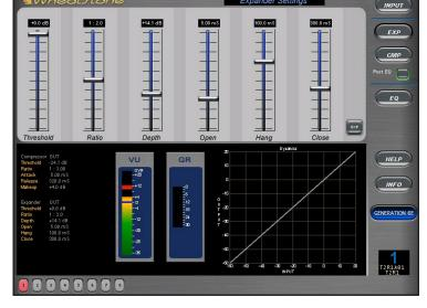
unlike nearly any other processing element it is active - i.e. working, attenuating away the input signal - when the input signal is at its quietest, at or below the threshold. If the expander is on, there will be gain reduction when no signal is present. The gain-reduction reduces as the threshold is approached, and there is none above the threshold.
