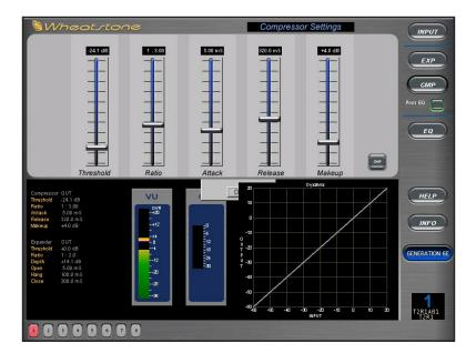
RATIO (1:1.00 - 1:20.0) — The proportion by which a signal exceeding the threshold is reduced in level. "1:3" means that a change in signal level above the threshold by 15dB will be reduced to only a 5dB change in level.
